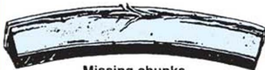
Missing chunks and separating layers
